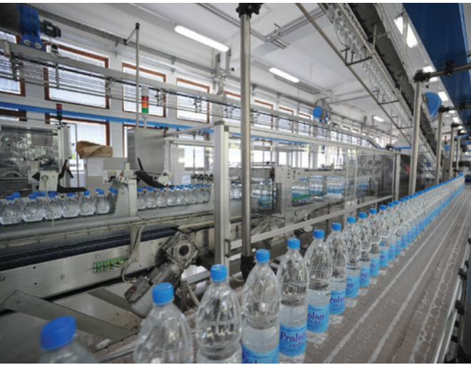
Proton water in bottles with blow-fill-cap technology proceed along an assembly line. Photo courtesy of Sidel
