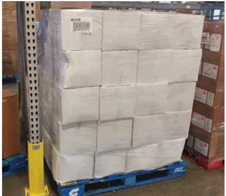
When not fully encased, such as with metal cans on trays, there is an increased propensity to denting and scuffing due to the inherent elements of the LTL environment. Photo courtesy of NMFTA
