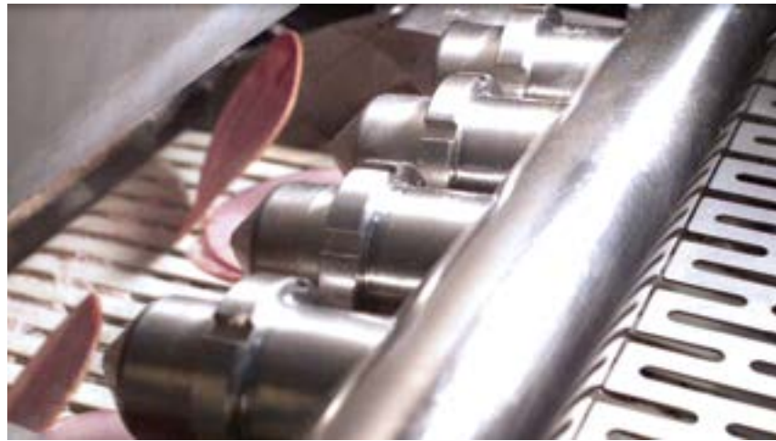
Sonotek applies edible coatings to frozen foods to reduce freezer burn.
