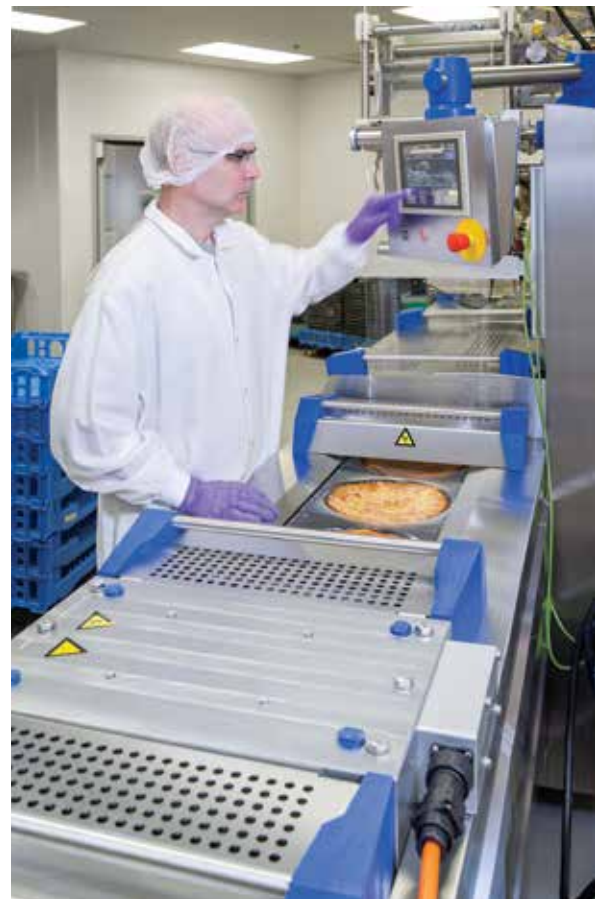
The Reiser horizontal form-fill-seal packaging machine produces vacuum, MAP, and VSP packages to reduce oxidation in foods such as pizza. Photo courtesy of Reiser
