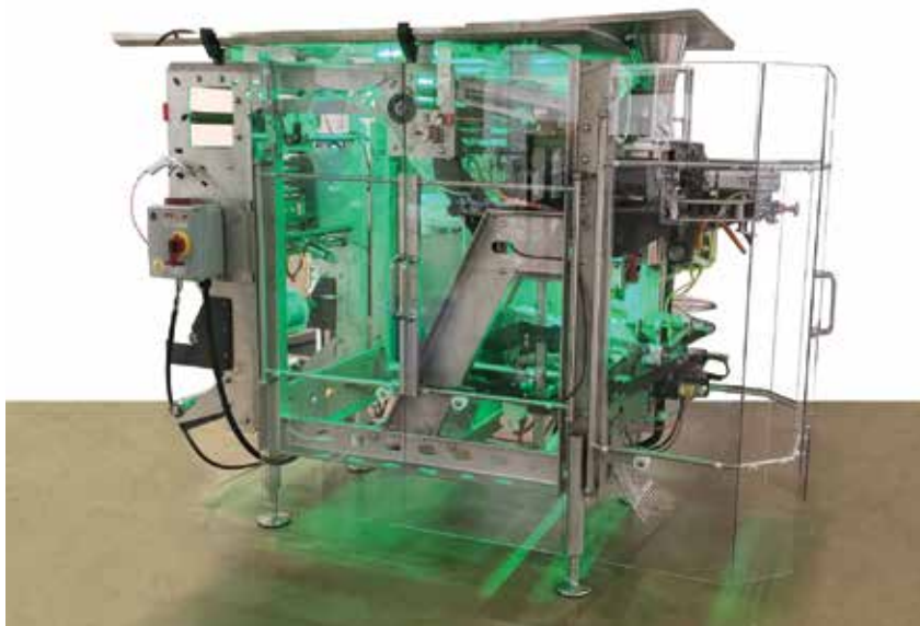
The BW Flexible Systems ISB family of vertical form-fill machines reduces O_2 to levels ranging from 1% to 2% for foods prone to oxidation, such as cheese and chips. Photo courtesy of BW Flexible Systems
